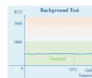
Automatic temperature control in the measuring chamber can keep a stable background value, not affe by the ambient temperature, ensuring the accuracy of measurement results.
