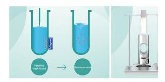
Magnetic separation washing and non-contact vortex mi units, with different mixing modes depending on differen assays, ensuring a sufficient washing to reduce the non-specific binding.
