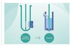
In the wash station, four waste liquid needles are equipped with four independent washing units to avoid the carry-over.
